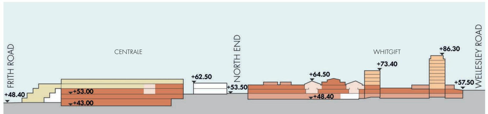
Fig 34 Section 2 from Frith Road to Wellesley Road, cutting across the more central part of both Whitgift and Centrale Shopping Centres with a total change in level of approximately 9m from west to east
